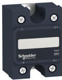
single phase relay, Harmony Solid State Relays, 125A, panel mount, zero voltage switching, thermal pad, input 4 to 32V DC, output 48 to 660V AC
