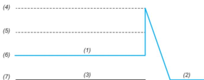
Overvoltage range : 26...36 VDC, Latch Mode
