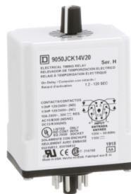
Timing Relay, Type JCK, plug In, on delay, adjustable time, 1.2 to 120 seconds, 10A, 240 VAC, 120 VAC/110 VDC
