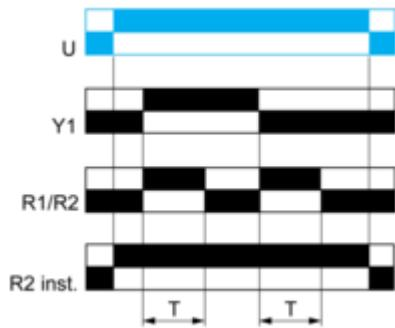
**Function C : Off-Delay Relay with Control Signal**
