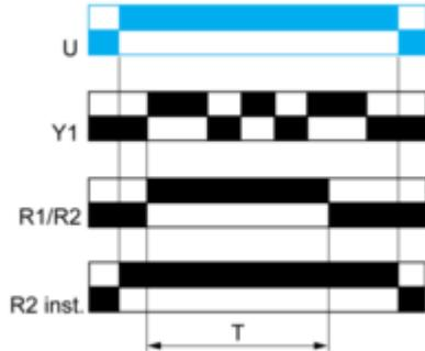
**Function Bw : Double Interval Relay with Control Signal**
