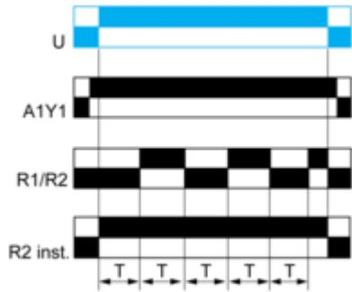
Before power-up Y1 should be permanently connected to A1.
