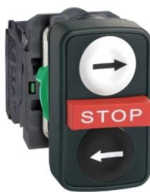
Triple headed push button, Harmony XB5, XB4, white flush, red projecting, black flush pushbutton, 22 mm, spring return, 2NO + 1NC
