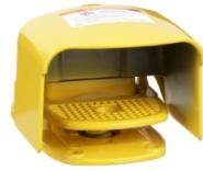
Foot Switch, Harmony 9002AW, industrial, pedal and side shields, SPDT contact, NEMA 2, 4, 13 enclosure, 5A resistive at 600V AC
