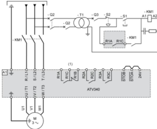
(1) : Use relay output R1 set to operating state Fault to switch Off the product once an error is detected.
