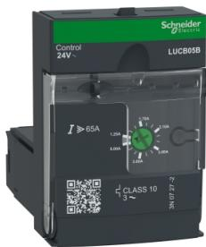
Advanced control unit, TeSys Ultra, 1.25A to 5A, 3P motors, protection & diagnostic, class 10, coil 24VAC
