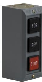
Push button, Type B, standard duty control station, 5A, 600 VAC, FORWARD/REVERSE/STOP, NEMA 1
