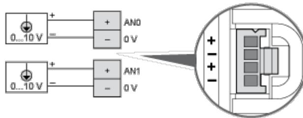
The (-) poles are connected internally.
