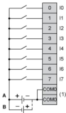
(1) The COM0 terminals are connected internally.
