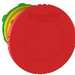
Emergency stop head, Harmony XB5, switching off, plastic, red mushroom 40mm, 22mm, trigger and latching turn to release
