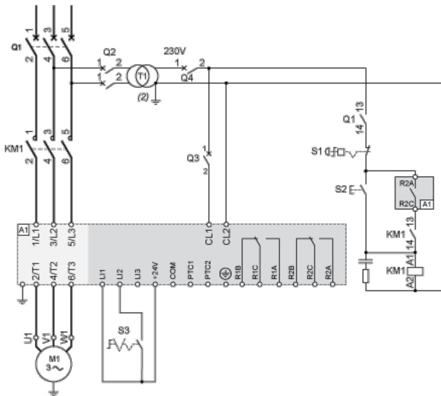
**Connection in the motor delta winding in series with each winding****Wiring**
