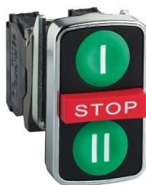
Triple headed push button, Harmony XB4, metal, 22mm, marked, 1 green flush I + 1 red projecting STOP + 1 green flush II, 2 NO + 1 NC
