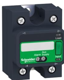
Harmony, Solid state relay, 75 A, DIN rail mount, zero voltage switching, thermal pad and smart diagnostic, input 4...32 V DC, output 48...660 V AC
