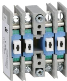
Adder deck, Harmony 8501X, screw clamp terminals, 10A resistive at 600V AC, 4NO, 4 standard contact cartridges
