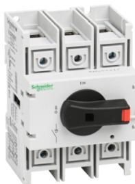
Disconnect switch, TeSys VLS, body switch, 80A, 40HP at 480VAC, UL98, three phase, 100kA SCCR, size 2, DIN rail mount
