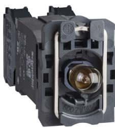
Complete body/contact assembly and light block, Harmony XB5, XB4, with body/fixing collar, BA9s incandescent bulb, 110...120V, 1NO + 1NC
