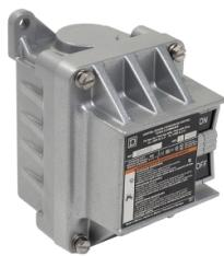
Complete control station, Harmony 9001B, 2 push buttons ON/OFF, Maintained Contact, 5A, 600V AC, 2NO, NEMA 7/9
