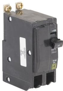
Mini circuit breaker, QO, 50A, 2 pole, 120/240VAC, 10kA, bolt on
