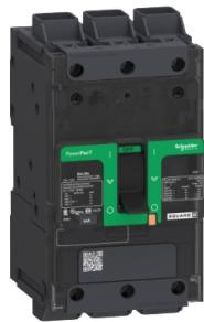
Circuit breaker, PowerPact B, 60A, 3 pole, 600Y/347VAC, 14kA, lugs, thermal magnetic, 80%
