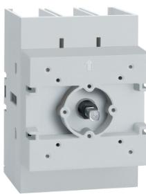
Disconnect switch, TeSys VLS, body switch, 30A, 20HP at 480VAC, UL98, three phase, 100kA SCCR, size 2, door mount
