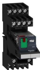
miniature pre assembled plug in relay with socket, Harmony Electromechanical Relays, 6A, 4CO, lockable test button, mixed terminal, 24V AC
