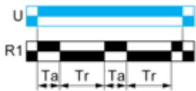
**Function Lt: Asymmetrical Flashing Relay (Starting Pulse Off) & with Pause / Summation Control****Description**
