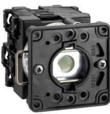
Cam switch body for BCD encoded without output switch, Harmony K, 22mm, plastic, 1 pole, 11 positions, 45 degree, 12A
