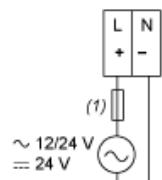
(1) Type T fuse (Controller: 1.25 A, Expansion: 1 A)
