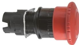
Head for emergency stop push button, Harmony XB6, red mushroom 30mm, 16mm, trigger latching turn to release, unmarked
