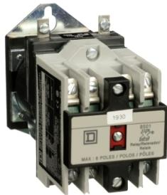
NEMA Control Relay, Type X, machine tool, 10A resistive at 600 VAC, 4 normally open contacts, 115/125 VDC coil, pan head
