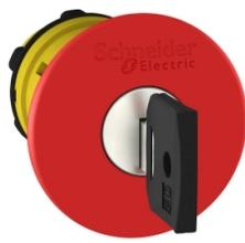
Head for emergency stop push button, Harmony XB5, switching off, plastic, red mushroom 40mm, 22mm, trigger/latching key release, key 458A
