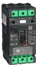
**Motor Circuit Protector, TeSys BV4, high fault, 7A, 600Y/347 VAC, 42 to 98 instantaneous trip, up to 100kA SCCR**
