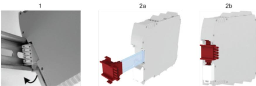
1 : Mount controller CPU and modules on rail.
