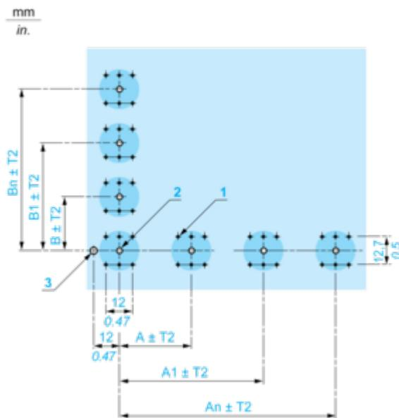
A 24 mm/0.94 in. minimum for rectangular heads, 18 mm/0.71 in. minimum for square or circular heads
