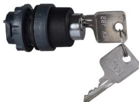
Key switch selector head, Harmony XB5, plastic, black, 22mm, key 4A185, 3 positions, push turn to release
