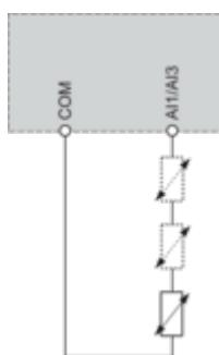
It is possible to connect either 1 or 3 sensors on terminals AI1 or AI3
