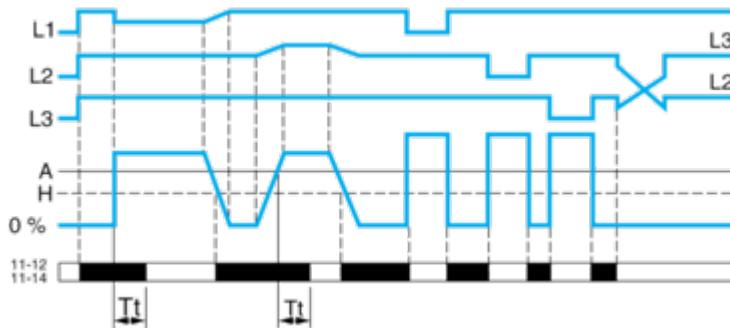
**Control of Overvoltage and Undervoltage in Window Mode**
