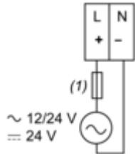
(1) Type T fuse (Controller: 1.25 A , Expansion: 1 A)
