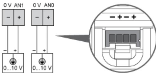
The (-) poles are connected internally.
