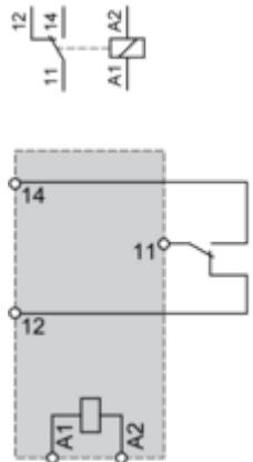
**NOTE:** For DC input, A1 have to be +, otherwise it would short circuit from protection module
