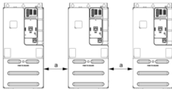
$a \geq 50 \text{ mm (1.97 in.)}$  from  $50\text{...}60^{\circ}\text{C}$ , no restriction below  $50^{\circ}\text{C}$
