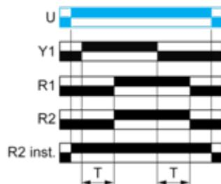
Function Act: On-Delay & Off-Delay with Control Signal & With Pause / Summation Control**Description**
