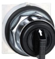
Head for selector switch, Harmony 9001K, metal, standard handle, black, 30mm, 3 positions, stay put, Cam C
