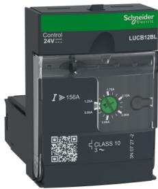
Advanced control unit, TeSys Ultra, 3A to 12A, 3P motors, protection & diagnostic, class 10, coil 24VDC
