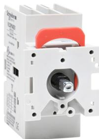
Disconnect switch, TeSys VLS, body switch, 40A, 20HP at 480VAC, UL508, three phase, 5kA SCCR, size 1, door mount
