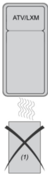
(1) Braking resistor
