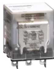
Plug in relay, Type R, miniature, 1 HP at 277 VAC, 15A resistive at 120 VAC, 11 blade, 3PDT, 3 NO, 3 NC, 24 VAC coil
