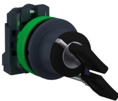
Selector switch, Harmony XB5, flush mounted sw. key 455 2 pos stay put key release L/R 1 NO screw
