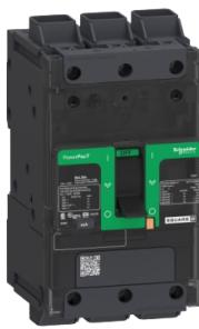
Circuit breaker, PowerPact B, 70A, 3 pole, 600Y/347VAC, 14kA, lugs, thermal magnetic, 80%
