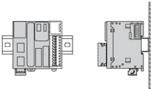
**Acceptable Mounting Position**
