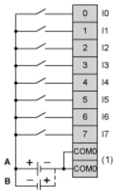
(1) The COM0 terminals are connected internally.
