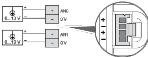
The (-) poles are connected internally.
