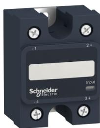
single phase relay, Harmony Solid State Relays, 10A, panel mount, zero voltage switching, thermal pad, input 3 to 32V DC, output 24 to 300V AC
