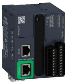
logic controller, Modicon M221, 16 IO, 8 DI, 8 DO, transistor, PNP, Ethernet
