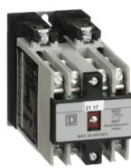
NEMA Control Relay, Type X, master, 10A resistive at 600VAC, 6 normally open contacts, 110/120VAC 50/60Hz coil
